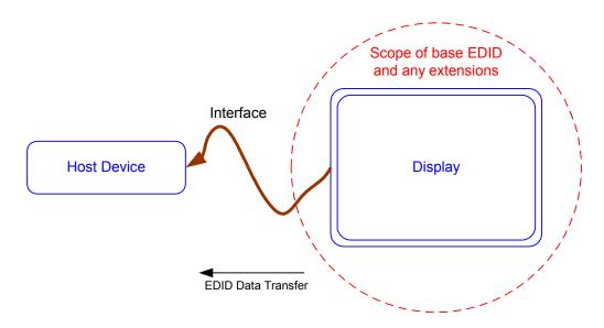
**Note:** Generally the display identified above will be a product connected to a host (source) via an external interface. However, in some cases products with an embedded display may use EDID, in which case the display above may be a subsystem of the product with an internal interface to the control (host) subsystem.
