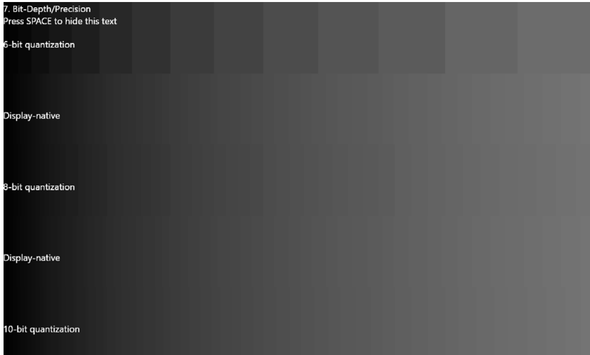
Figure 7-1: Gradient Ramp Bars to Illustrate Simulated Bit Depth
