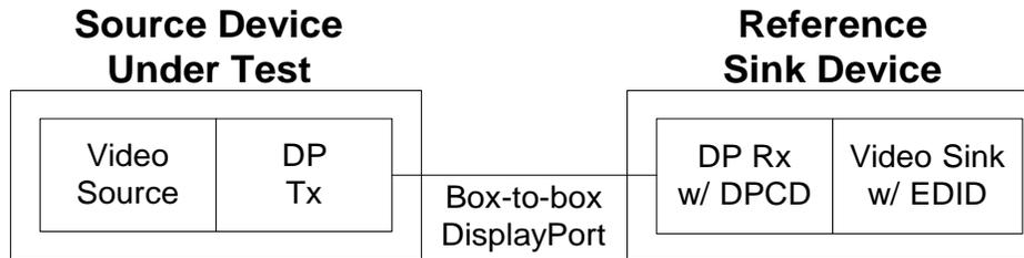
**Figure 4-1: Source Device Compliance Test Setup for Link Layer and Above**
