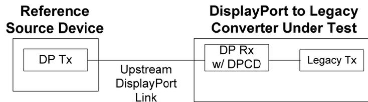
**Figure 6-2: DisplayPort to Legacy Converter Compliance Test Setup**
