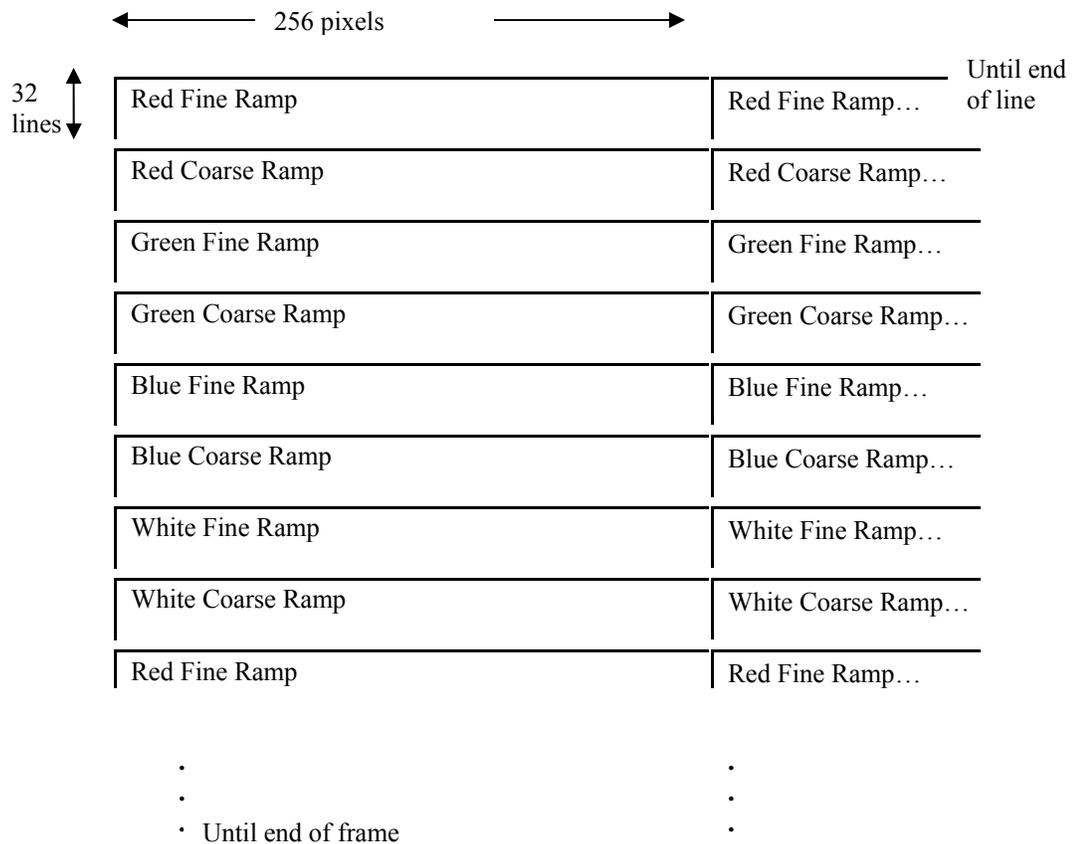
**Figure 3-2: Color Ramp Test Pattern (Two Ramps per Color)**
