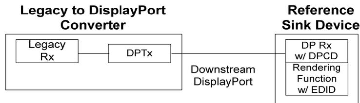
**Figure 6-1: Legacy to DisplayPort Converter Compliance Test Setup**
